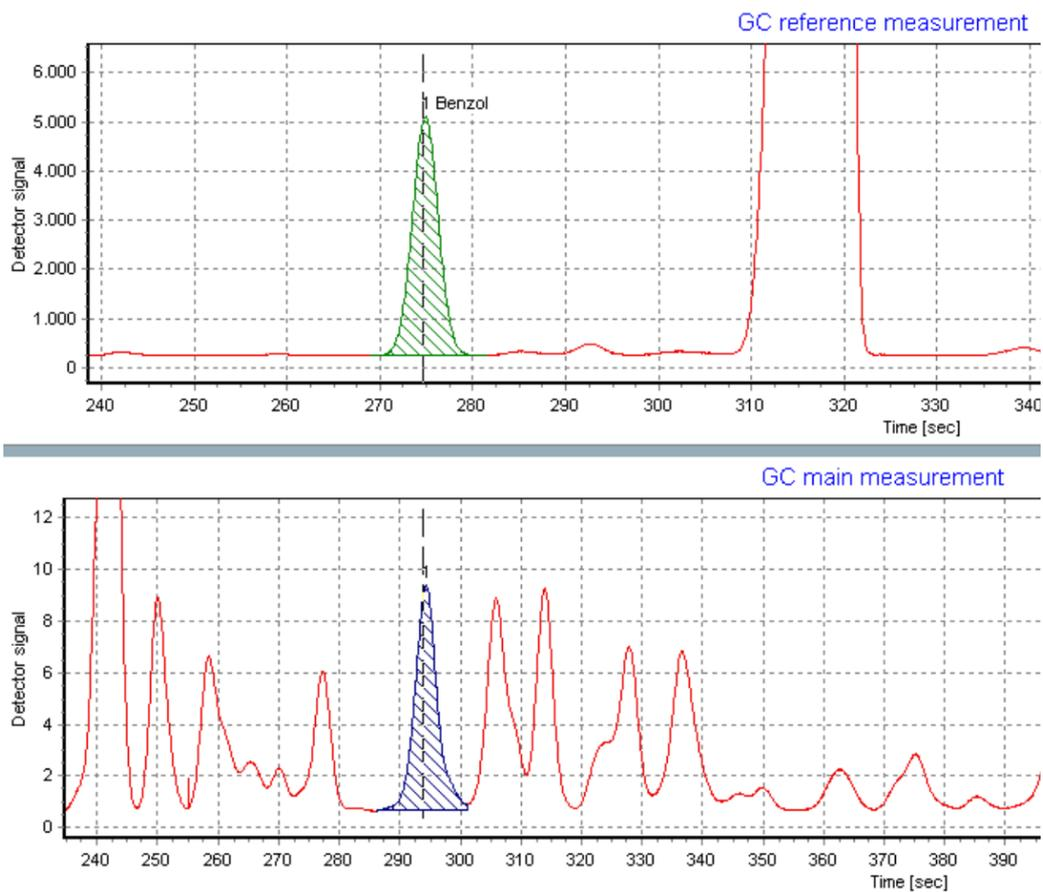
Fig. 17: Comparing reference measurement and main measurement
