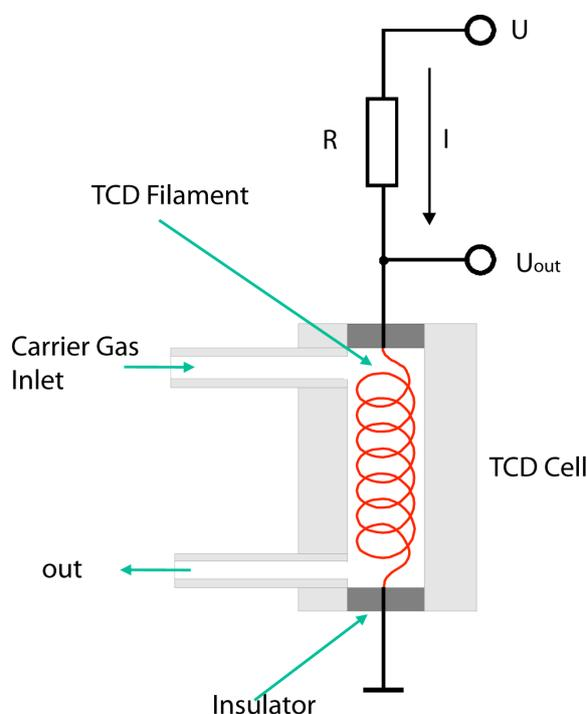
Fig. 26: Principle of the TCD
