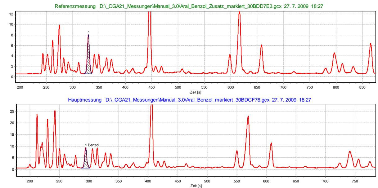
Fig. 13: Comparison of gasoline and gasoline with benzene added
