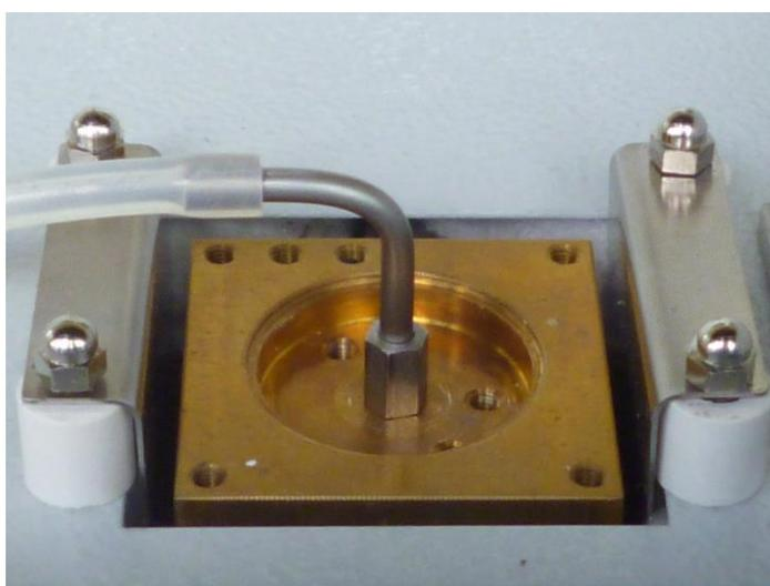
Fig. 35: Measuring hydrogen and carrier gas flow at the FID
