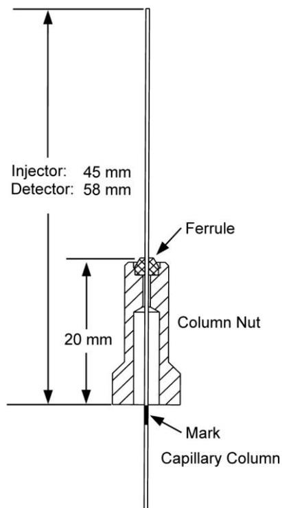
*Fig. 36: Preparations when installing the capillary column*
