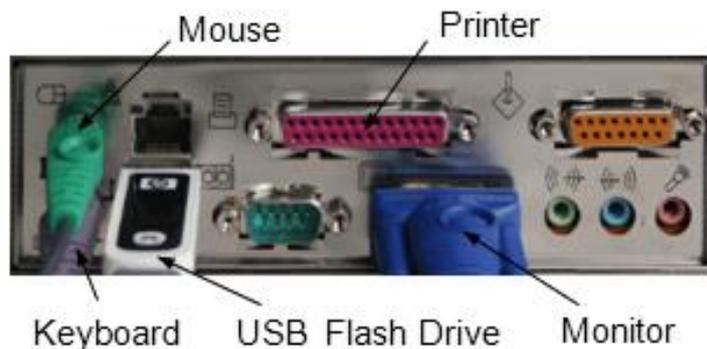
Fig. 1 Connector panel
