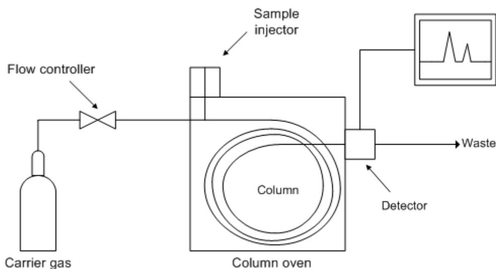
Fig. 18: The operating principle of a gas chromatograph (Wikipedia)
