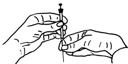
Fig.11: Inserting the needle into the injector
