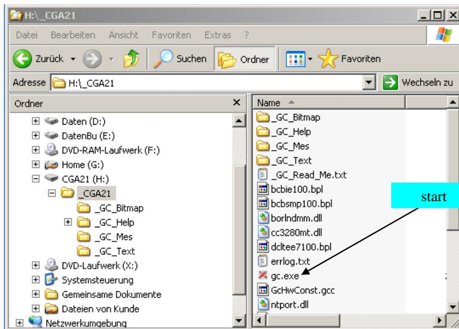
Fig. 10: Starting the software on a workstation
