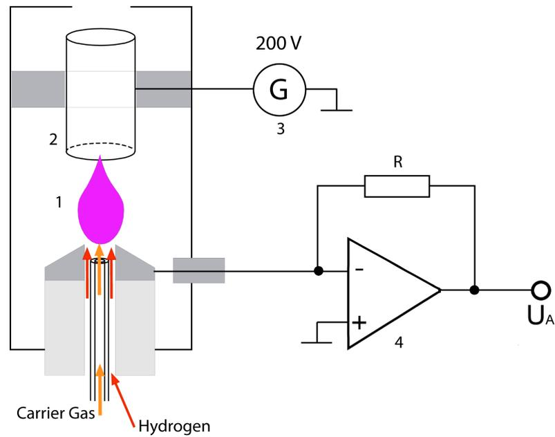
Fig.29: Technical design of the FID
