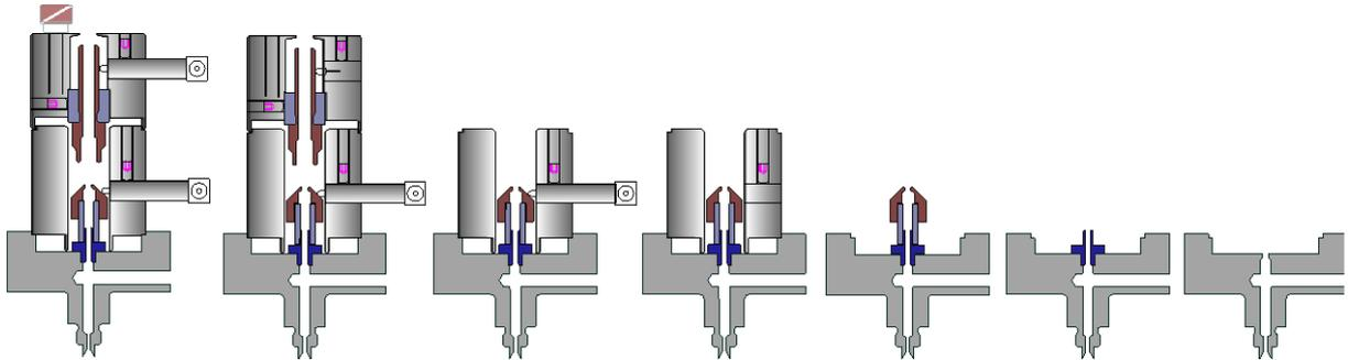
Fig. 32: Disassembling the FID
