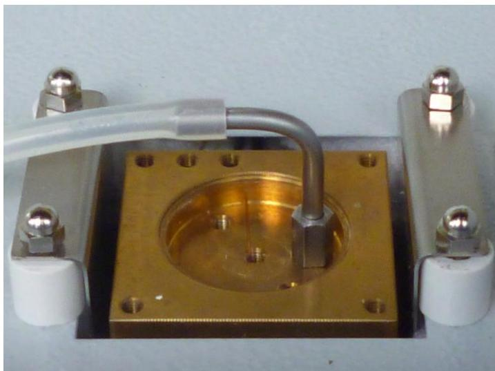
Fig. 34: Measuring air flow at the FID
