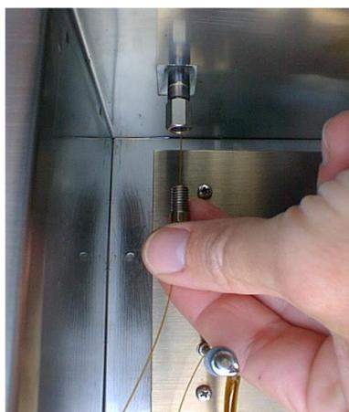
*Fig. 37: Connecting the column on the injector side*
