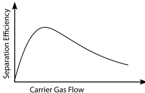
*Fig.30: Separation efficiency vs. gas flow*
