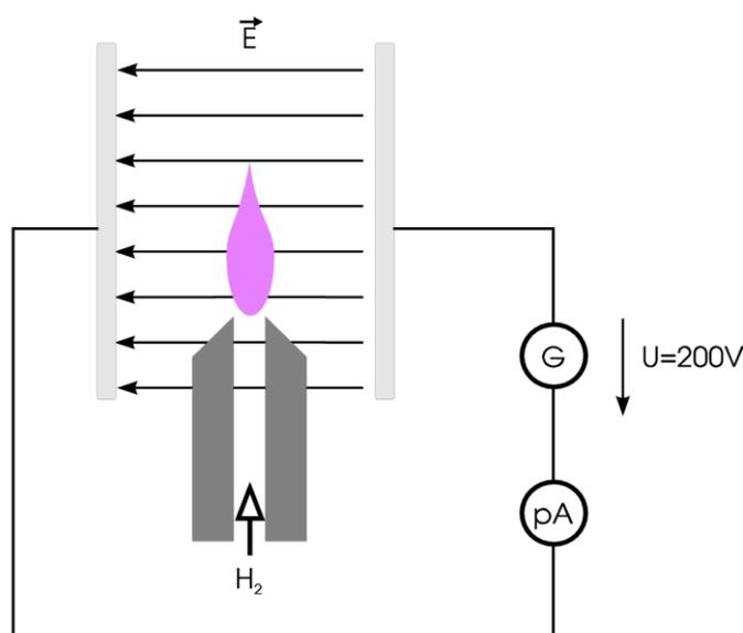
Fig.28: Operating principle of the FID
