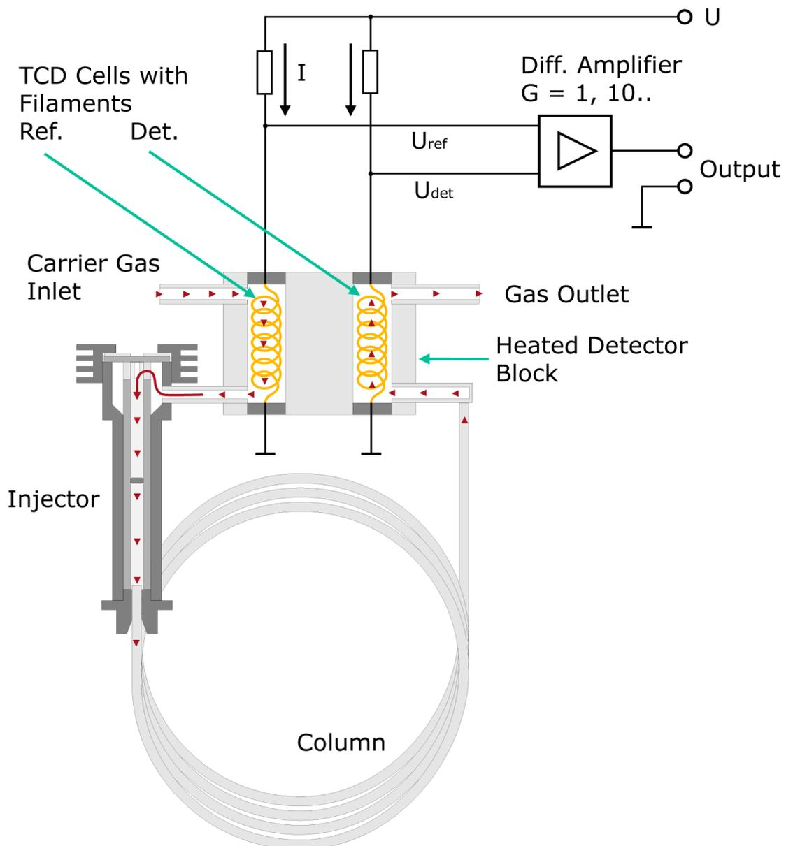
Fig. 27: Realisation of TCD with reference cell
